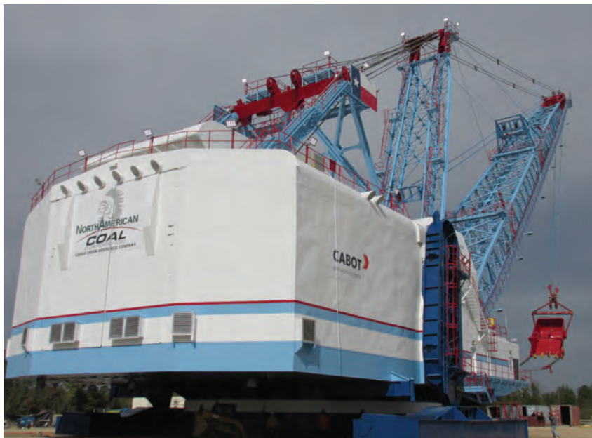
The revolving frame deck was expanded with transformer extensions on the left and right sides of the machine behind the propel girders, making the machine broader across the back.
