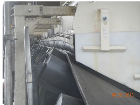
New Parallel Conveyors Replacing Troublesome Crossover Conveyors in Coal Transfer House
